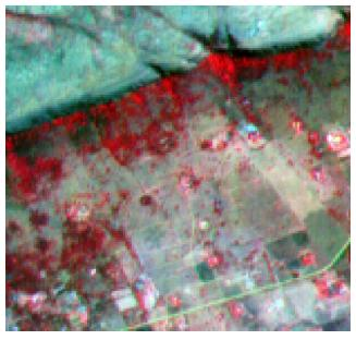
Same image area after the Forward FFT (Fast Fourier Transform) and Destripe procedures were run on the individual bands. Striping has been completely suppressed with no blurring or degradation of ground features.
