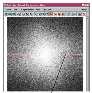
The Manual Destriping mode was used to process the ASTER image shown here. In this mode the Parameters window lets you outline areas in the FFT (Fast Fourier Transform) raster representing the striping frequencies, and define the amount of suppression to apply to them. A Test option lets you preview the destripe result for your designated sample area.
