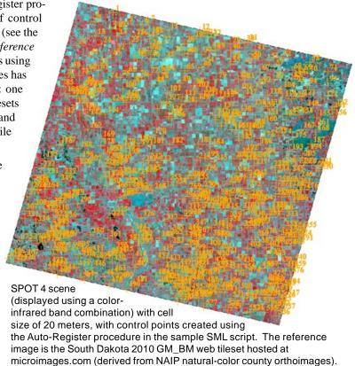
so no selection filter is required. The resulting pipeline stages for the input image and reference are passed as parameters to the Run() method of the AUTOREGISTER class, which carries out the operation and creates the resulting control-point georeference in memory. A Save() method on the class is then used to write this georeference subobject to each of the bands of the input image.
