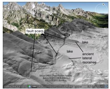
Shaded-relief Google Earth 3D tilesett showing a fault scarp along the eastern foot of the Grand Teton mountain range, Wyoming. Terrain and shading created from Lidar DEM with 0.5-meter cell size.
