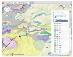
Geomashup of geologic map data layers that includes an SVG geometric tileset, three KML geometric tilesets, and a KML file.
