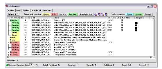
The TNTmips Job Manager window opens automatically (if not already open) when new job files are created. It allows you to select pending jobs and change their status (hold, release, delete, or set to run with the next available processor thread) and shows run times and progress bars for current running jobs. Lists of completed and failed jobs are shown on separate tabbed panels. You can also set up time and day-of-week scheduling for jobs.
