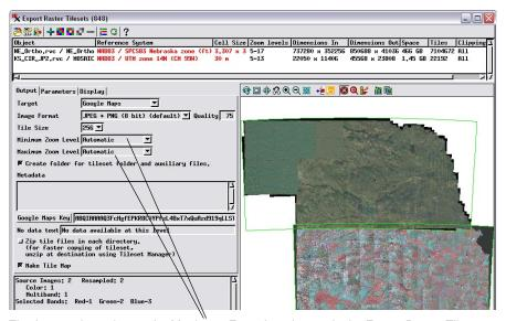
The Automatic setting on the Maximum Zoom Level menu in the Export Raster Tilesets window sets an appropriate maximum zoom level individually for each of the output tilesets based on the cell size of the input image. Likewise, the Automatic setting on the Minimum Zoom Level menu automatically sets an appropriate minimum zoom level for each tileset based on its maximum zoom level and aerial extents.
