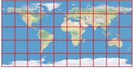
Left, table showing range of possible prerendered, fixed zoom levels in a NASA World Wind tileset. World Wind uses an equirectangular (Plate Carree) earth model and a tile size of 512 pixels. Its lowest zoom level is a 5 x 10 array of tiles with each tile covering 36 degrees of latitude and longitude, as shown in the illustration above. Each subsequent zoom level doubles the number of tiles in both directions, as in Google Maps and Bing Maps.
